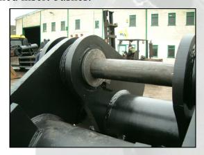
They are also available for quick hitch mounting but be aware this does reduce the crushing force! They mount directly to the end of the dipper and link as with a bucket and then have a brace arm which pins to the underside of the dipper using a brace pad (supplied) to hold the fixed half in place
