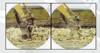
The lower crushing legs and toeplates are manufactured completely from Hardox 400 and 450 type material for strength and for increased attachment life
