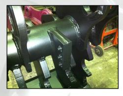
All pulverizers for machines 13 ton and upwards include rebar cutters in the throat.
