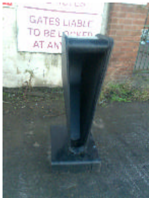
Tapered digging buckets for laying small pipes for 1 to 13 ton machines
