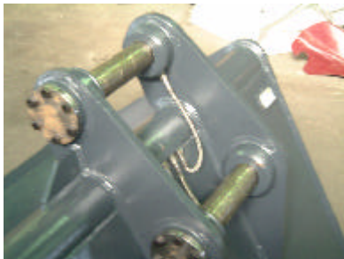
Sealed pin buckets for long reach dredging machines working under water etc.
