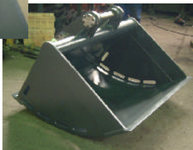
Sealed pin buckets for long reach dredging machines working under water etc.
