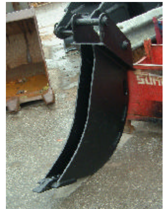
Deep dig buckets for cable laying etc
