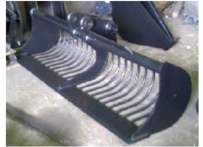
Reed buckets with round bars in the floor for drainage work
