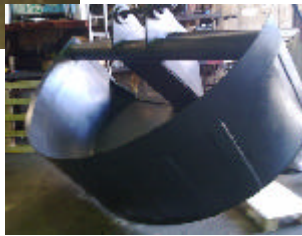
Curved bottom trenching buckets for pipe laying
