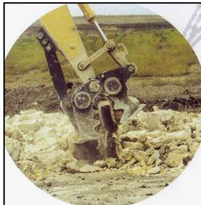
The lower crushing legs and toeplates are manufactured completely from Hardox 400 and 450 type material for strength and for increased attachment life
