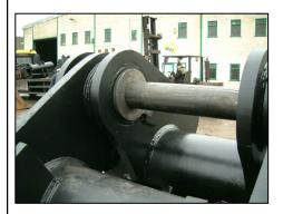
The Pulverisor hinges on the main dipper pin and comes complete with a longer hardened main pin.
